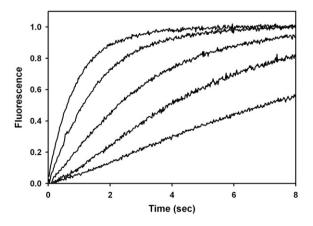
**Fig. 4.** Effect of temperature on bicelle–nanolipoprotein particle mixing kinetics. Temperatures, from upper to lower curves: 33.2, 30.0, 26.8, 23.6, and 20.5 °C. Same concentration conditions as lower curve in Fig. 1.
