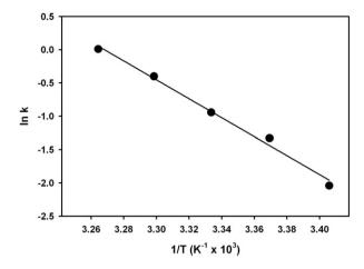
**Fig. 5.** Arrhenius plot of kinetic constants. Data in Fig. 4 fit with Eq. (1) to obtain pseudo-first-order rate constants.
