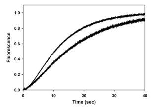
**Fig. 3.** Effect of added apolipoprotein (MSP1E3D1). Lower curve, 2.8  $\mu$ M nanolipoprotein particles (5.6  $\mu$ M MSP1E3D1). Upper curve, additional 14  $\mu$ M MSP1E3D1 added. Bicelle 1,2-dimyristoyl-sn-glycero-3-phosphocholine (DMPC) = 15 mM (about 125  $\mu$ M bicelles, assuming 120 DMPC/bicelle).
